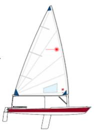
The Laser Radial sail is 62 square feet. The Radial sail and mast were created in the 1980s. Additional information about the Laser Class Association is at www.laser.org or www.nalaser.org
